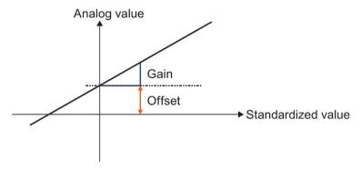
The straight line in the graphic describes which standardized value is being converted into which analog value. Gain corresponds to the slope of the straight line and offset to the movement of the zero point of the straight line on the y-axis.
