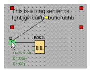
A linked comment moves consistently with the figure to which it is attached. You can adjust the relative position of the comment to the figure, as you do a block comment.
