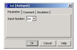
AS-Interface inputs are named Ia. The block number of an AS-Interface input is determined by the hardware structure.
