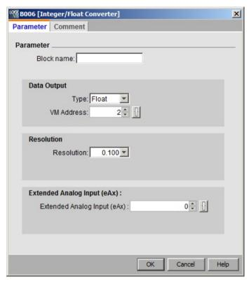
**Data Output**: The output of Integer/Float is stored in VM. You can chose the output type as float or double and the start VM address where the converted float stores.
