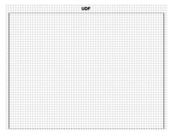
A UDF has a rectangle to indicate its edit area. You can edit the position and dimensions of this area.
