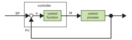
The comparing element and the controller function describe the conduct of the controller.
